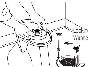
**IMPORTANT** Do not lift or rock the toilet after placement. A new gasket must be installed if the seal is broken.
